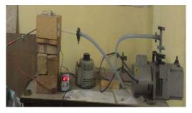
Muffle Furnace (~ 1200 °C)
