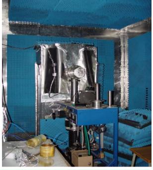
It has 250 kV, 2 kA, 150 ns electron facility developed locally first time in Indian University. Using this, 2 MW backward wave oscillator is developed for the first time in the country.
